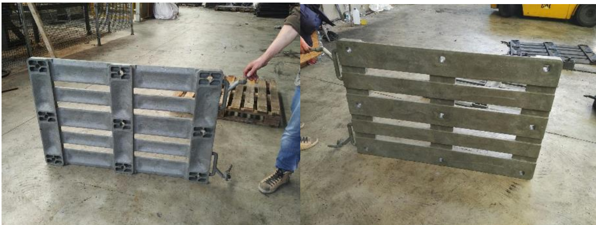
First board moulded during pre-tests at supplier: front and rear view
