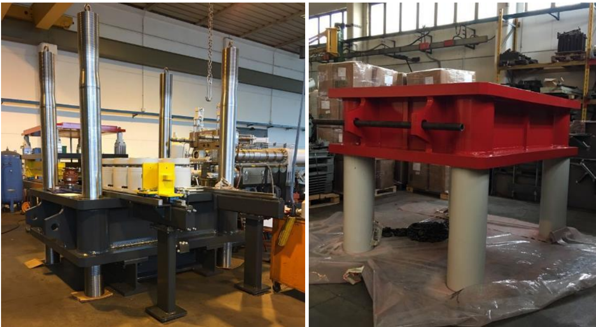
Left: Spacers and pistons installed on lower press; right: upper press.
