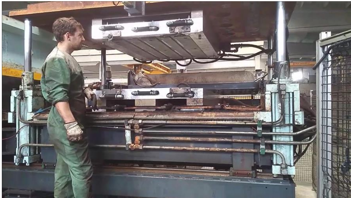
Pre-tests of pallet moulds at supplier
