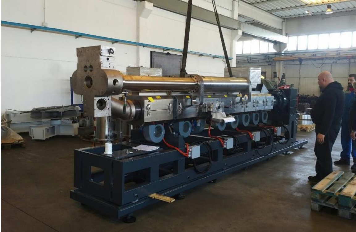
Installation of Injection unit on support.
