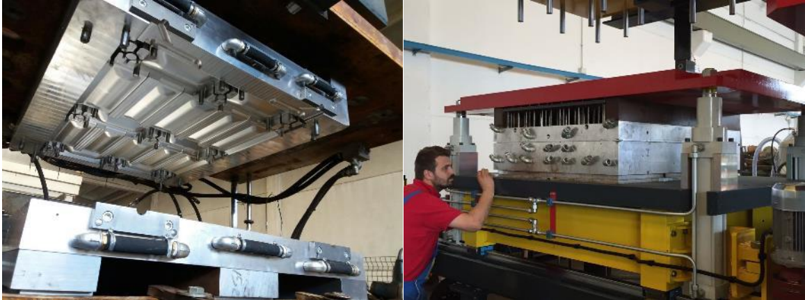
Moulds assembled on press for pre-tests at supplier
